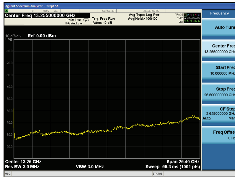
Figure 7-10. Rise in noise floor indicates changes in sensitivity with changes in LO harmonic used
