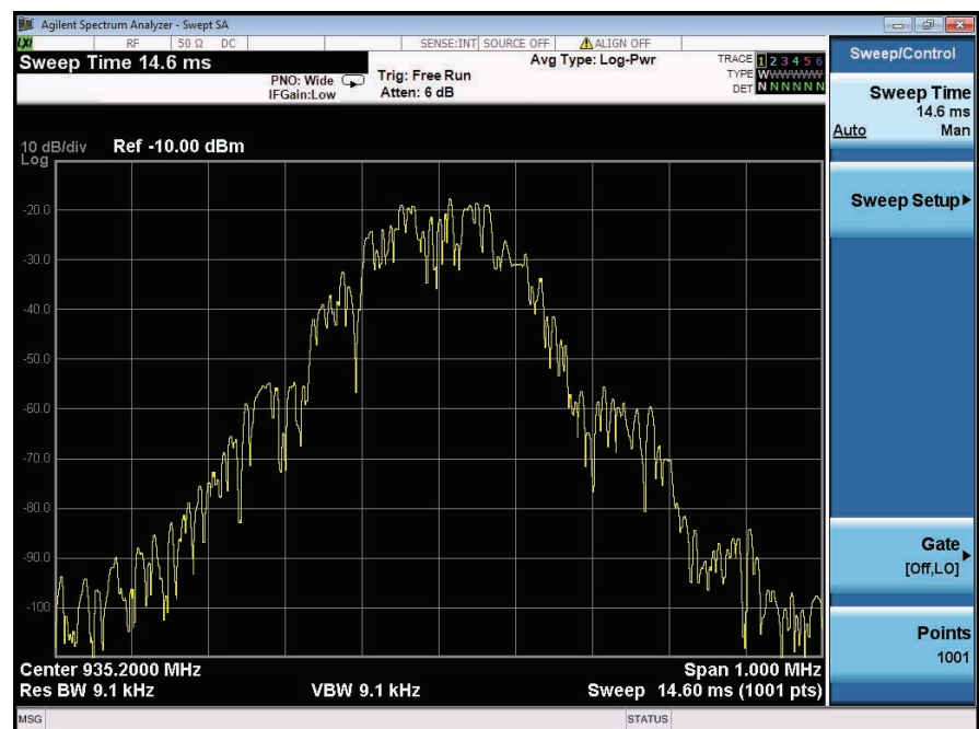
Figure 2-41. Spectrum of the GSM signal
